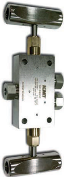
HP Stainless Steel Valve Assembly, 3-Way, 1 Press, .38, 2 Stem 60,000 psi
